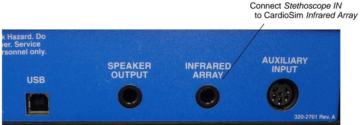
**Figure 12 Connecting SimulScope to CardioSim**
